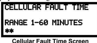
Select the number of minutes allowed, 1-60, before a fault is shown on the panel.
