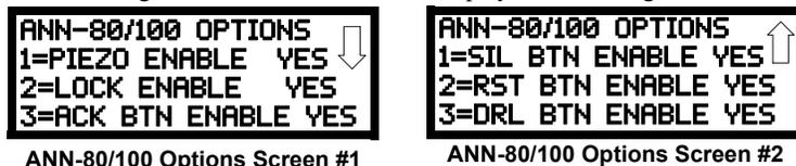
The *Piezo Enable* option allows the programmer to select whether the piezo sounder on any installed ANN-80 or ANN-100 module will ever sound. Pressing 1 while viewing the ANN-80/100 Options Screen #1 causes the display to toggle between *Piezo Enable Yes* and *Piezo Enable No*.
