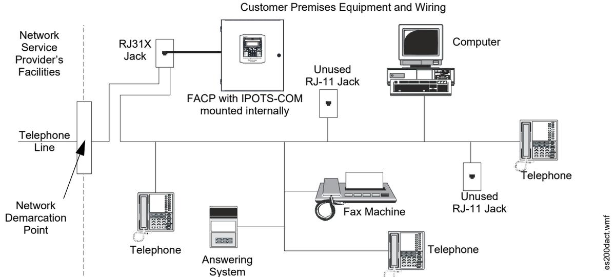
Figure 2.11 Communicator Installation
