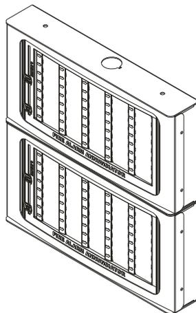
Figure 2.25 ANN-LEDs (shown in possible stacked configuration)
