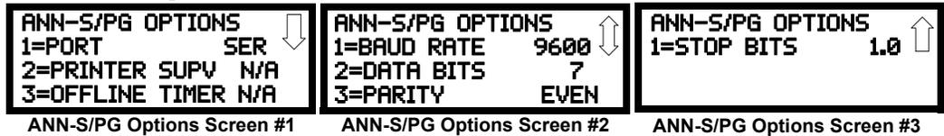
Pressing 1 for Port while viewing ANN-S/PG Options screen #1 will allow the programmer to select between a Parallel and Serial Port for printer connection. Each press of the 1 key will cause the display to toggle between *Port PAR* (parallel) and *Port SER* (serial). It is important to note that the interface selected determines which options are available to the user.
