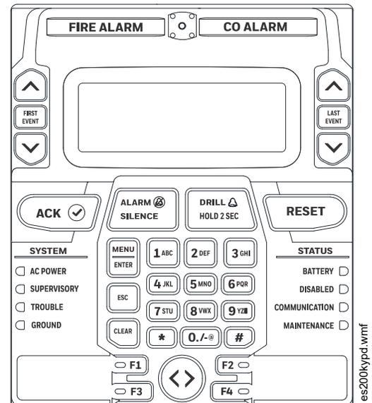
Figure 1.2 Membrane/Display Panel
