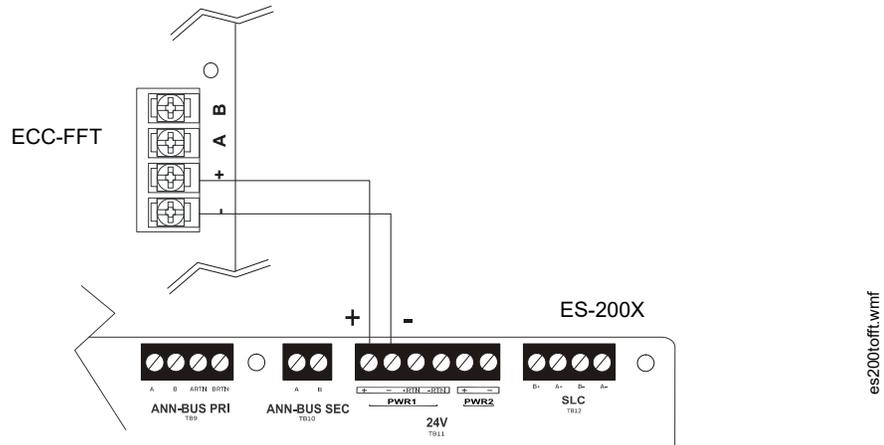
Figure 2.30 ECC-FFT Connections
