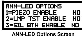
The *Piezo Enable* option allows the programmer to select whether the piezo sounder on any installed ANN-LED module will ever sound. Pressing 1 while viewing the ANN-LED Options Screen causes the display to toggle between *Piezo Enable Yes* and *Piezo Enable No*.
