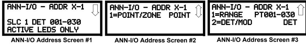
The first screen indicates that the ANN-I/O at ANN-BUS address 1 is programmed to annunciate SLC Loop #1 addressable Detectors with addresses 1 through 30. The programming can be changed using ANN-I/O Address Screens 2 and 3.
