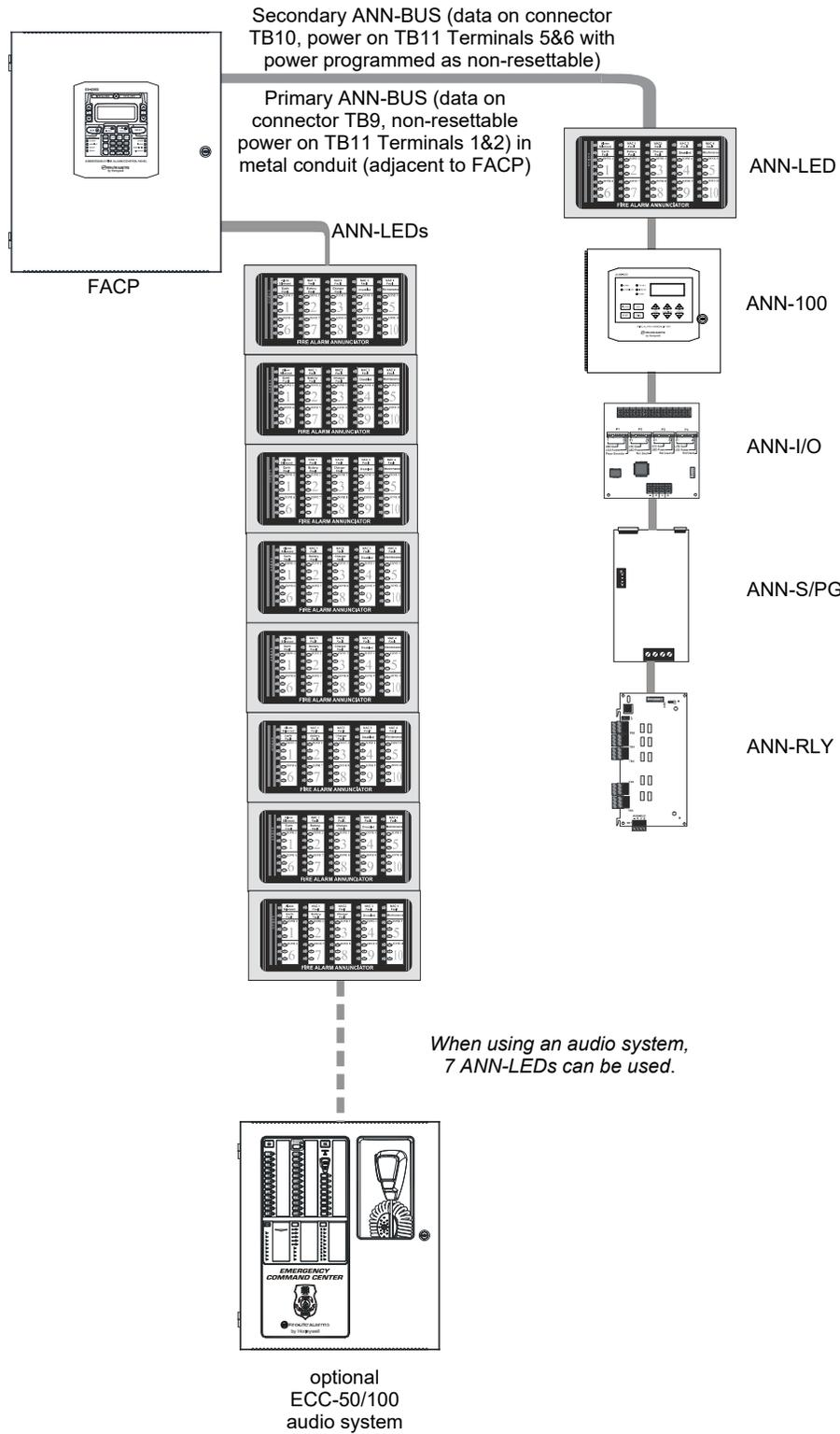
Figure J.2 FACP Maximum Configuration - Eight ANN-LEDs
