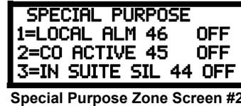
Zones 047, 048, 049, and 046 (and Zones 094 and 095 in Canadian mode) can be programmed for normal zone operation or for special purpose applications. In the above illustration, the four zones are shown Off, which means they can be programmed to function in the same manner as all other zones, by assigning them to input and output devices in the Programming Zone Assignment Screen.
