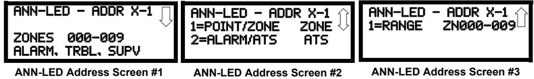
The first screen indicates that the ANN-LED at the selected ANN-BUS address is programmed to annunciate Alarms, Troubles and Supervisories for Zones 000 through 009. The programming can be changed using ANN-LED Address Screen 2.
