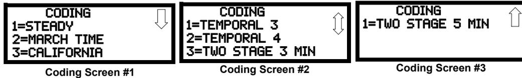
The programmer can select the notification appliance output by pressing the number corresponding to the desired output. The coding selections are:
