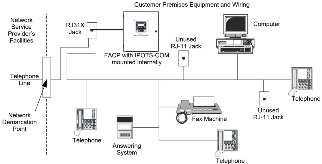
Figure 2.11 Communicator Installation
