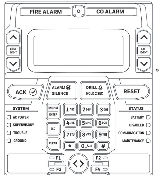
Figure 1.2 Membrane/Display Panel
