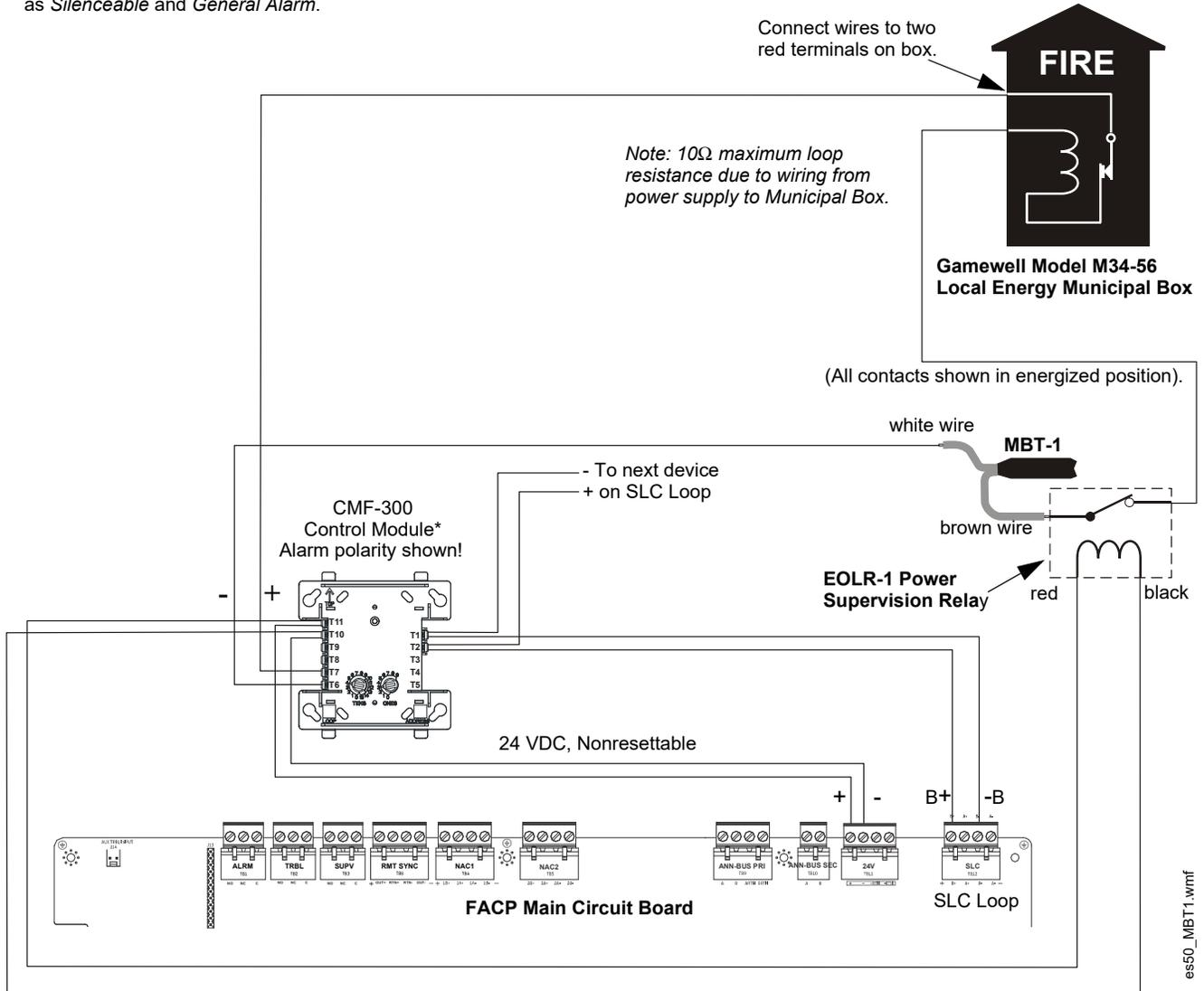
\*If the SLC device does not match the one in this figure, refer to the SLC manual wiring conversion charts for legacy and newer versions of the modules.
