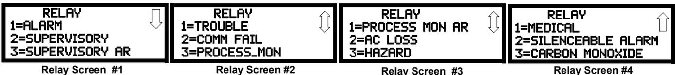
While viewing the selected screen, press the number corresponding to the desired relay type to program the main circuit board relay. The choice will be stored in memory and the display will return to the Relay Type Screen which will show the programmed type choice. Press the Escape key to return to the Relays Selection Screen and repeat the preceding procedure for the remaining relays.
