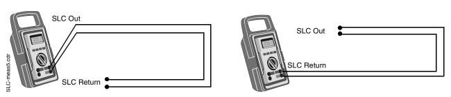
Figure 5.1 Measuring DC Resistance on an Unpopulated SLC Loop
