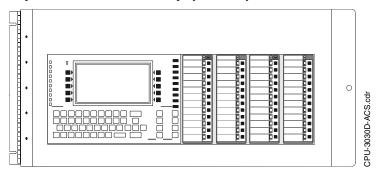
Figure 2.2 CPU2-3030D (Shown with Two Annunciators in DP-DISP)
