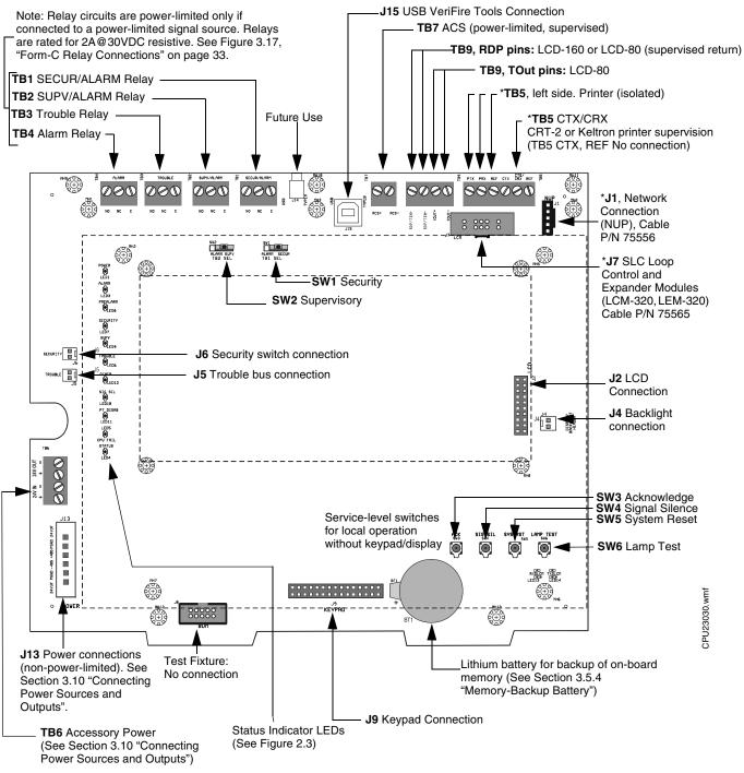
Note: Dotted line indicates location of optional keypad & LCD display
