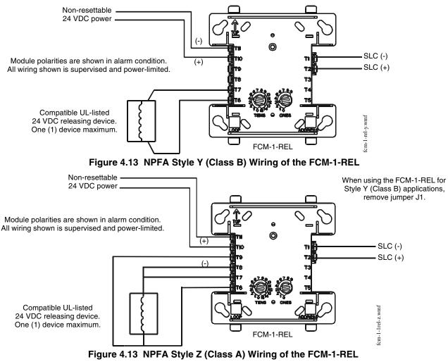
**NOTE:** With software version 14.0 or higher ALL new FlashScan Mode SLC releasing applications require the FCM-1-REL control module. The V-type FCM-1 control module may be used in SLC releasing applications with software version 14.0 or higher. H-type FCM-1 control modules do not support FlashScan mode releasing applications with software version 14.0 or higher. Use H-type FCM-1 for CLIP mode SLC releasing applications.
