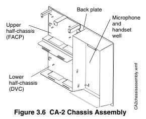
The NFS2-3030 mounts in the upper half-chassis. (Refer to Figure 3.6 and Figure 3.7.) If first mounting an optional LCM-320/LEM-320 pair behind the FACP, refer to Section 3.8.2, "Audio Applications with Chassis CA-2". Mount the NFS2-3030 to its half-chassis without removing the half-chassis from the back plate. Refer to "Memory-Backup Battery" on page 25 for removal of insulator.
