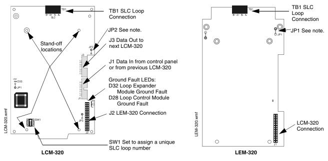
Note: Do not cut any jumpers on the LCM-320 or LEM-320.
