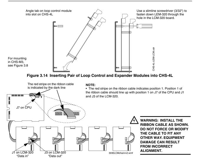
Figure 3.15 Connecting Multiple Pairs of Loop Control and Expander Modules
