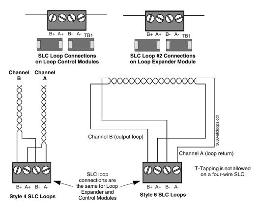
Figure 3.23 SLC Loop Connections and Wiring
