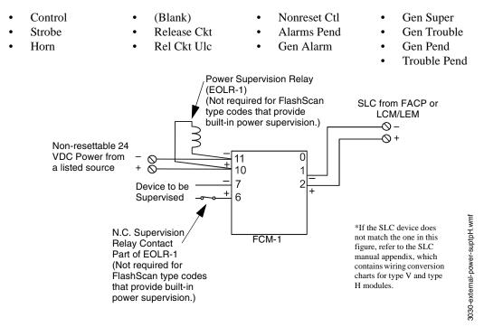
Figure 4.1 Enabling External Power Supervision Using Relays
