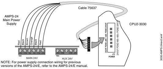
Figure 3.18 DC Power Connections: Main Power Supply
