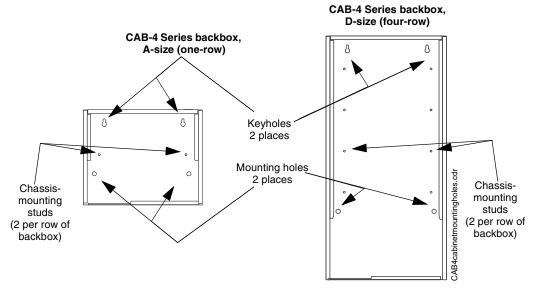
Figure 3.1 Backbox-Mounting Holes and Chassis-Mounting Studs
