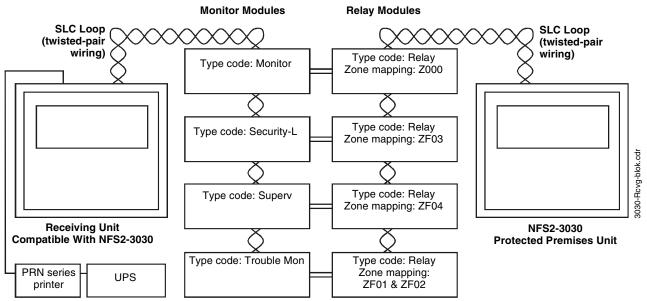
Note: Remote printers require 120 VAC, 50/60Hz primary power. A secondary power source (battery backup) is not provided; the use of a separate Uninterruptable Power Supply (UPS) 50 watt minimum, UL-listed for Fire Protective Signaling is recommended. A UPS is required for NFPA 72 Proprietary Protected Premises Receiving Unit Applications.
