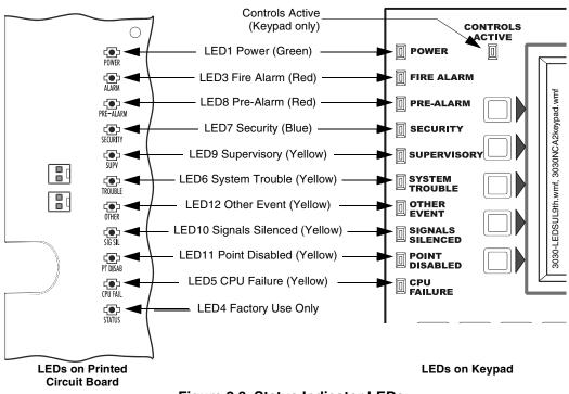
Figure 2.3 Status Indicator LEDs
