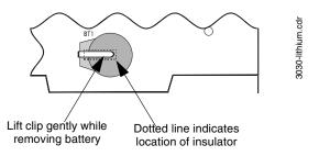
This battery's shelf-life should exceed 10 years, but if for some reason it fails, the control panel will show a trouble when powered up. To replace the lithium battery:
