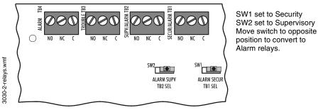
Figure 3.17 Form-C Relay Connections
