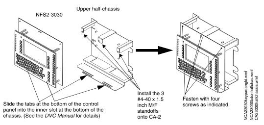
Figure 3.7 Mounting the NFS2-3030 onto the CA-2 Half-chassis
