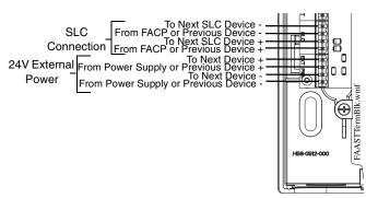
Figure 4.15 FSA-8000A Connection to the FACP
