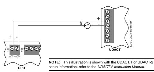
Figure 3.21 Wiring a Key Switch to Disconnect UDACT During Annual Testing
