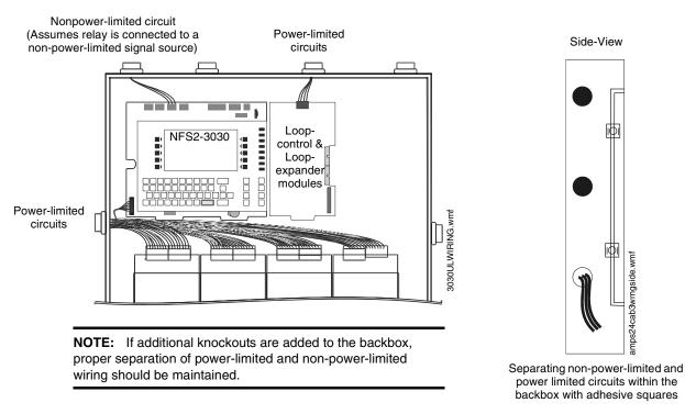
Figure 3.19 Typical Wiring in a Four-Row Backbox
