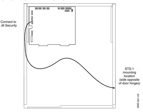
Figure 4.5 Installing the STS-1 Security Tamper Switch
