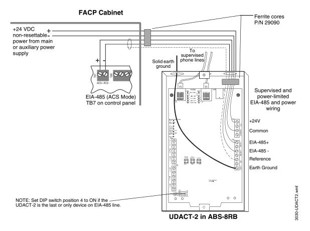
Typical wiring of a UDACT-2 with NFS2-3030:
