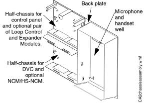
Figure 3.3 CA-2 Audio Chassis Assembly
