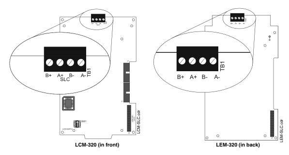
Figure 3.16 SLC Loop Connections on Loop-Control and Loop-Expander Modules
