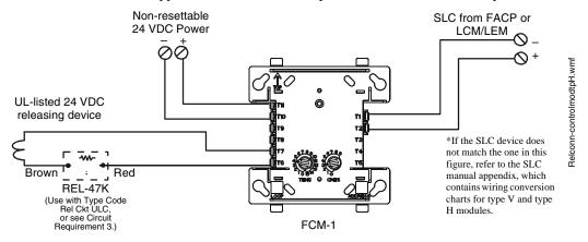
Note: See Circuit Requirements below. Devices for use in releasing applications **must** be programmed as type code RELEASE CIRCUIT or REL CKT ULC.
