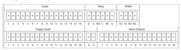
Table2: Z-Series Hybrid System auxiliary connections
